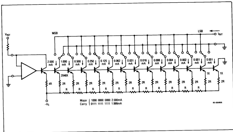
Figure 1. Traditional R-2R D/A Converter
