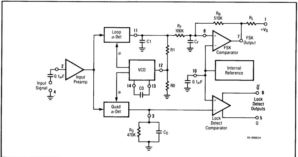
Figure 1. Generalized Circuit Connection for FSK and Tone Detection
