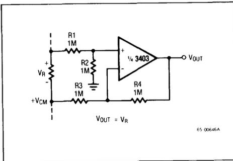
Figure 4. Ground Referencing a Differential Input Signal
