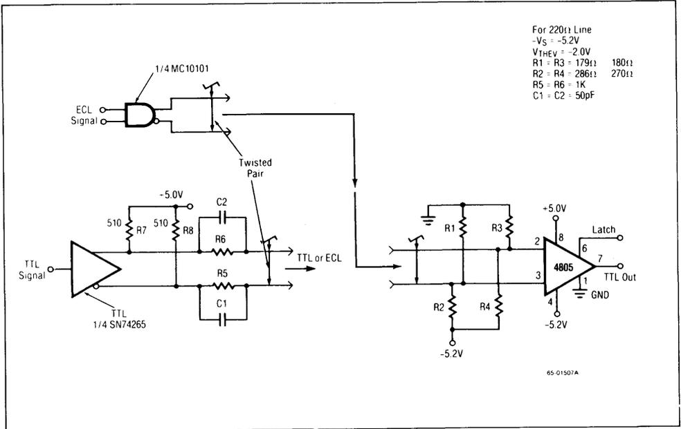
**Figure 7. Adaptive ECL-TTL to TTL Translator**
