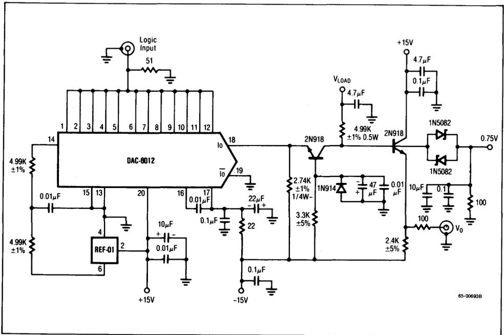
Figure 17. Settling Time Measurement Circuit
