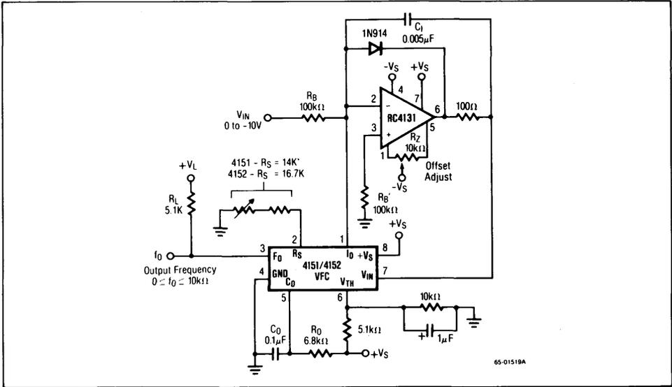
Figure 2. Precision Current — Sourced VFC
