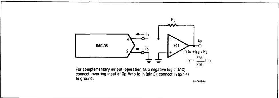
Figure 8. Positive Low Impedance Output Operation
