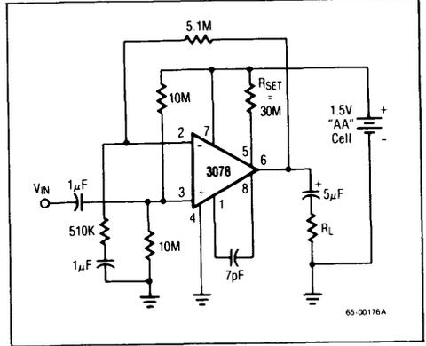
Figure 3. Non-Inverting 20dB Amplifier Circuit
