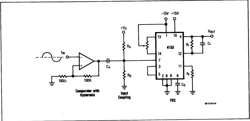
Figure 6. FVC Input Conditioning.
