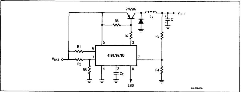
Figure 6. Complete Step-Down Regulator
