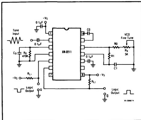
**Figure 4. Circuit Connection for Tone Detection**
