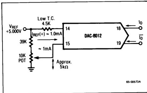
Figure 9. Recommended Full Scale
