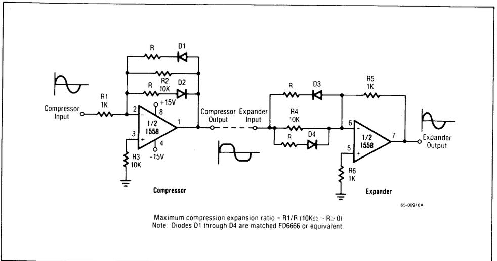
**Figure 4. Compressor/Expander Amplifiers**
