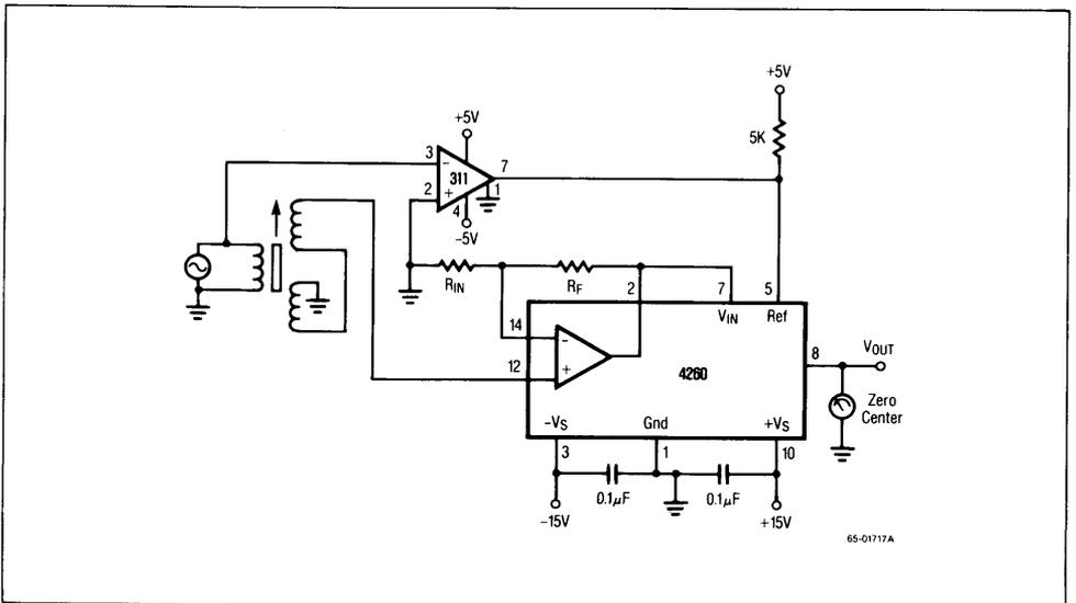
Figure 4. Linear Variable Differential Transformer With Phase Sensitive Detector
