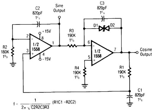
Figure 2. Quadrature Oscillator
