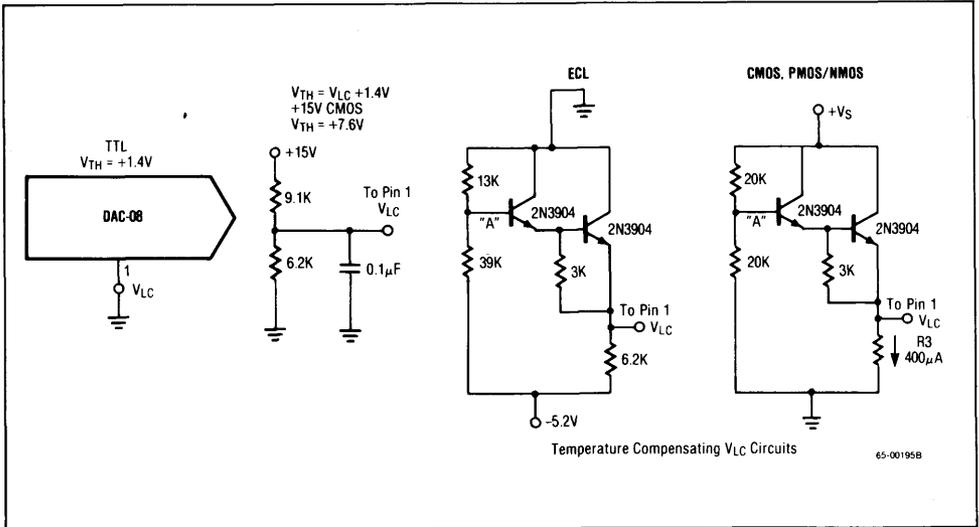
Temperature Compensating  $V_{LC}$  Circuits
