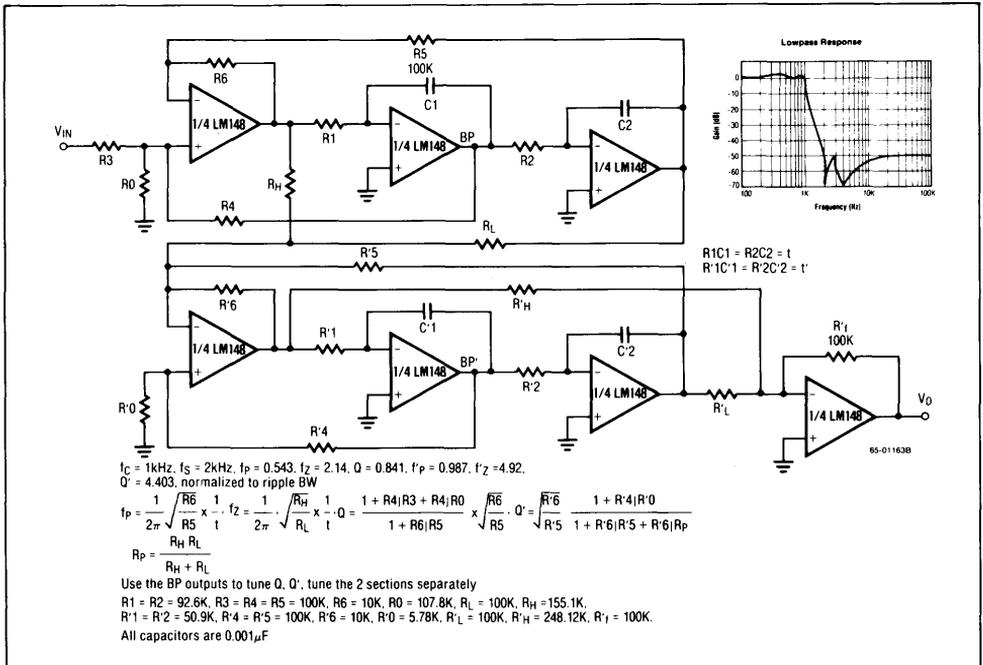
Figure 8. 4th Order 1 kHz Elliptic Filter (4 Poles, 4 Zeros)
