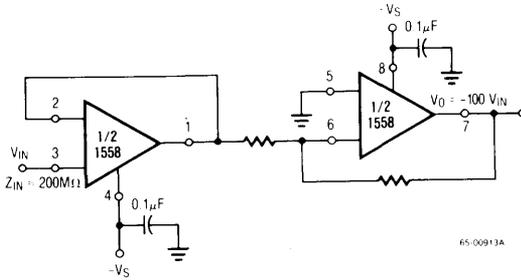
Figure 1. High-Impedance, High-Gain Inverting Amplifier
