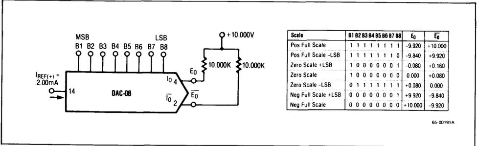
Figure 6. Basic Bipolar Output Operation
