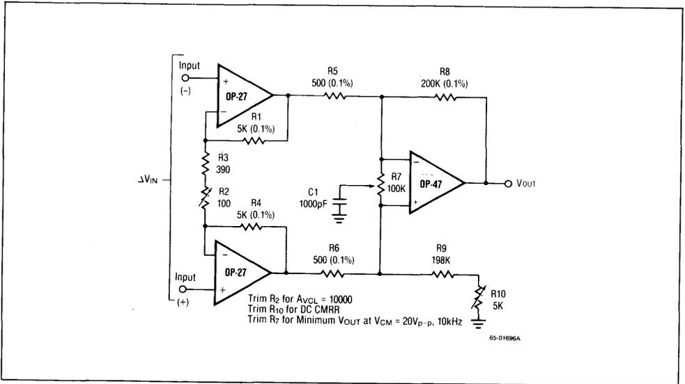
Figure 2. Three Op Amp IC Instrumentation Amplifier
