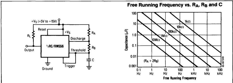
Figure 2. Free Running Operation
