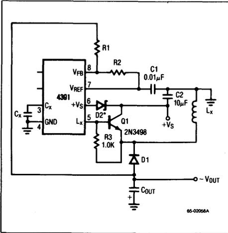
**Figure 5. High Voltage/High Power Application Circuit**
