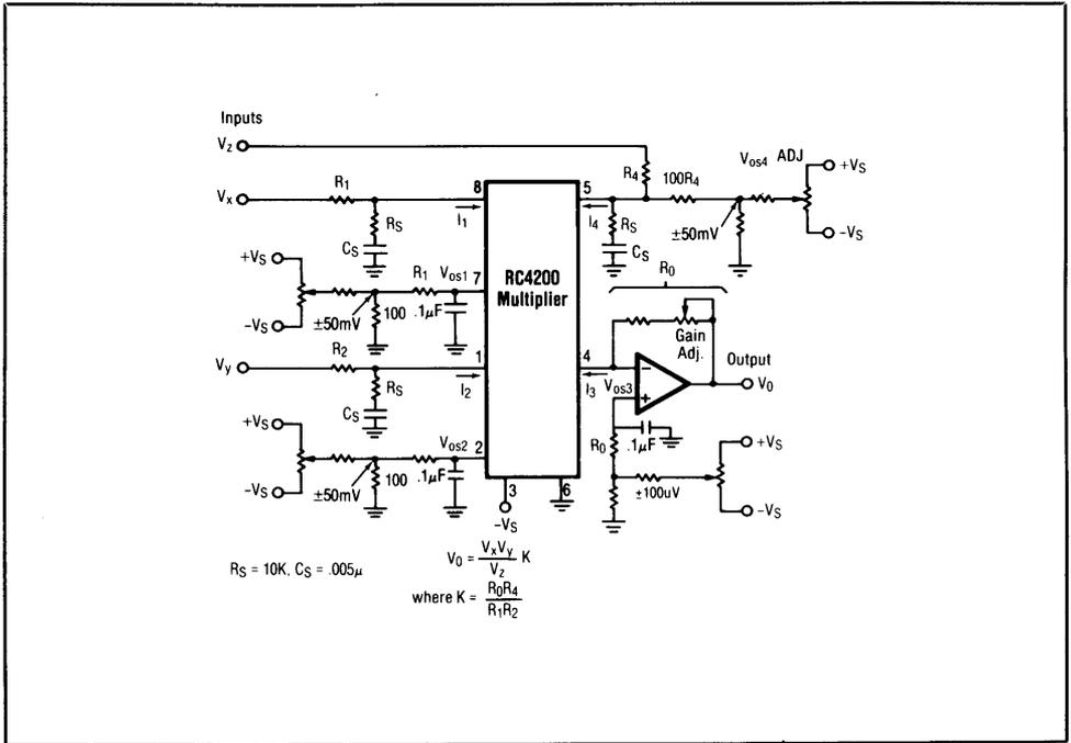
Figure 18. First Quadrant Multiplier/Divider
