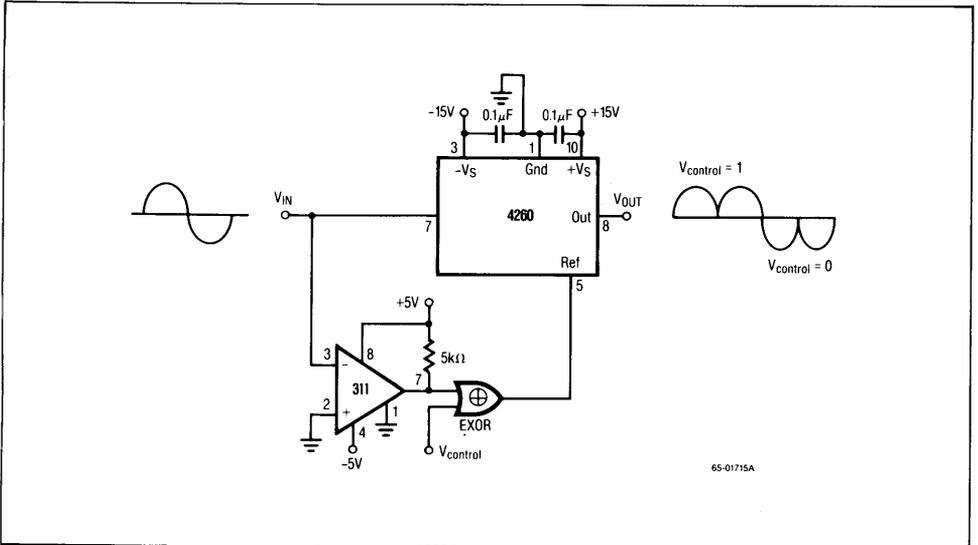
Figure 3. Precision Rectifier With Logic Switchable Output Polarity
