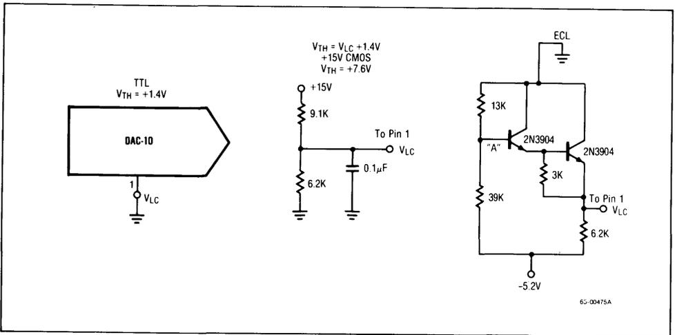
Figure 12. Interfacing With Various Logic Families
