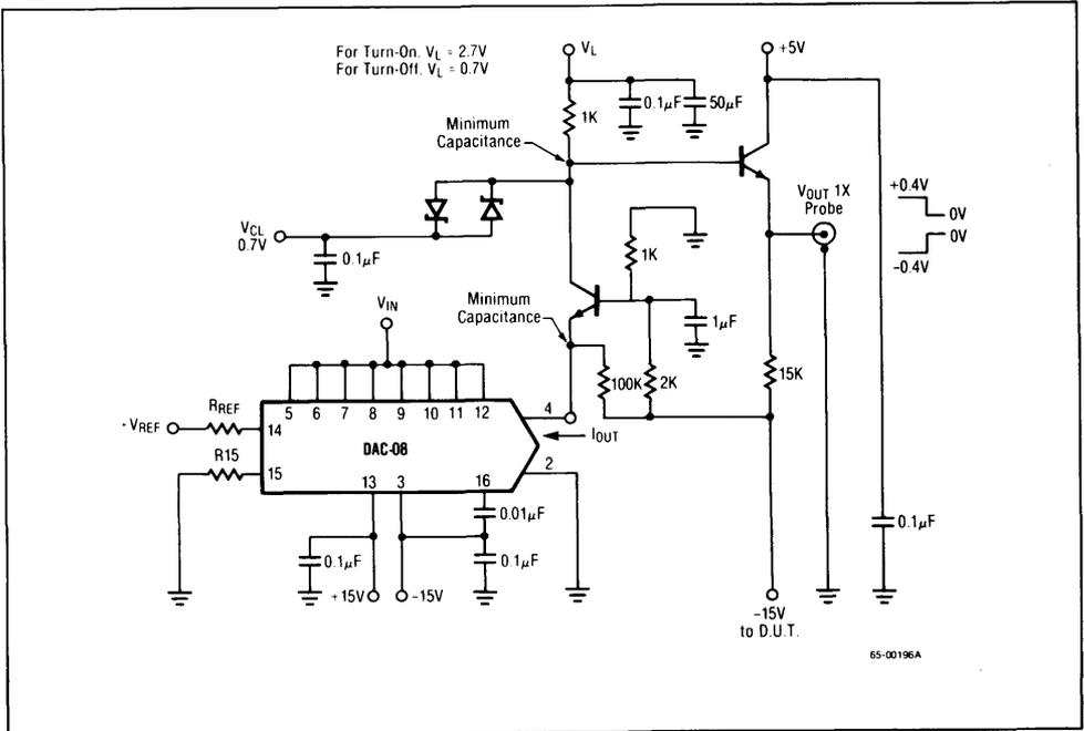
Figure 11. Settling Time Test Fixture
