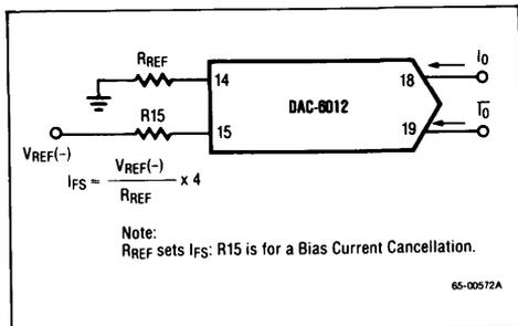
Figure 8. Basic Negative Reference Operation
