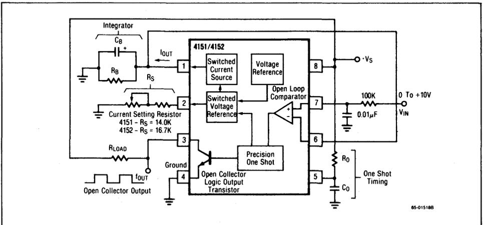
Figure 1. Single Supply VFC
