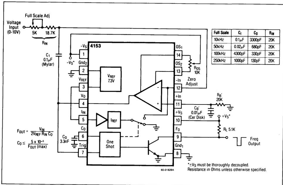
**Figure 3. Voltage-to-Frequency Converter With Offset and Gain Adjusts**
