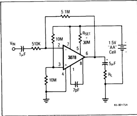
Figure 2. Inverting 20dB Amplifier Circuit
