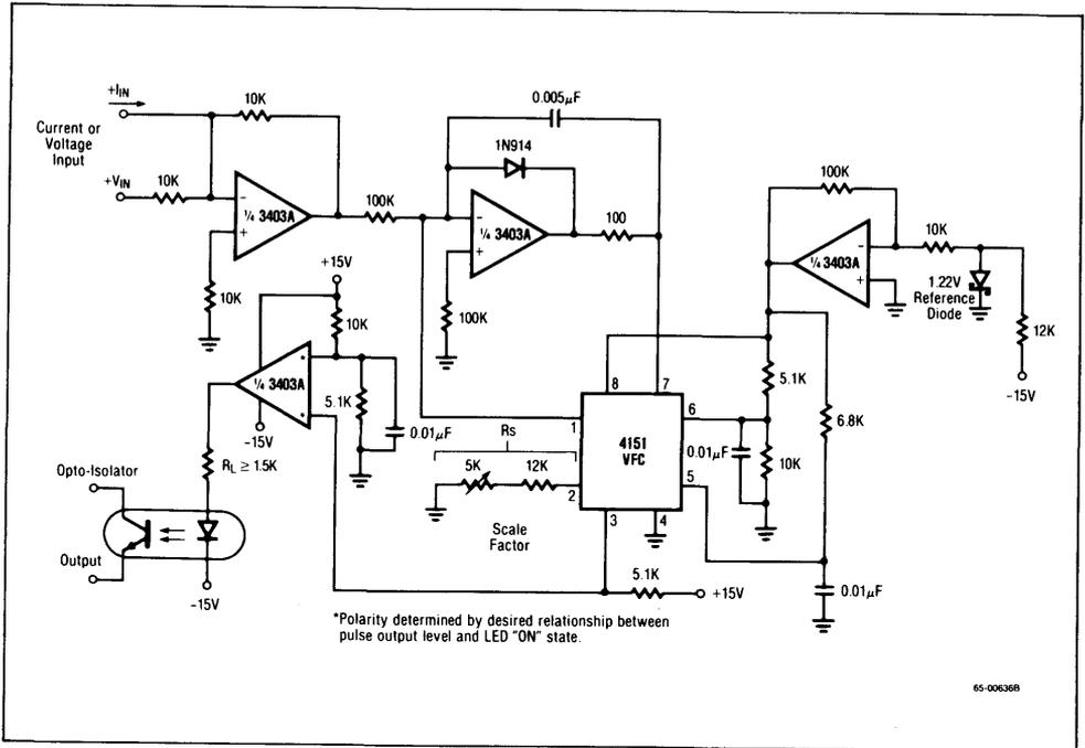
Figure 1. Precision Voltage-to-Frequency Converter With Isolated Output
