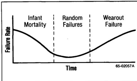
Figure 1. Failure vs. Time
