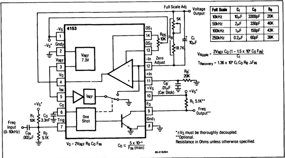
Figure 2. Frequency-to-Voltage Converter — V<sub>0</sub> (Volts) = F<sub>IN</sub> (kHz) — 100kHz Max
