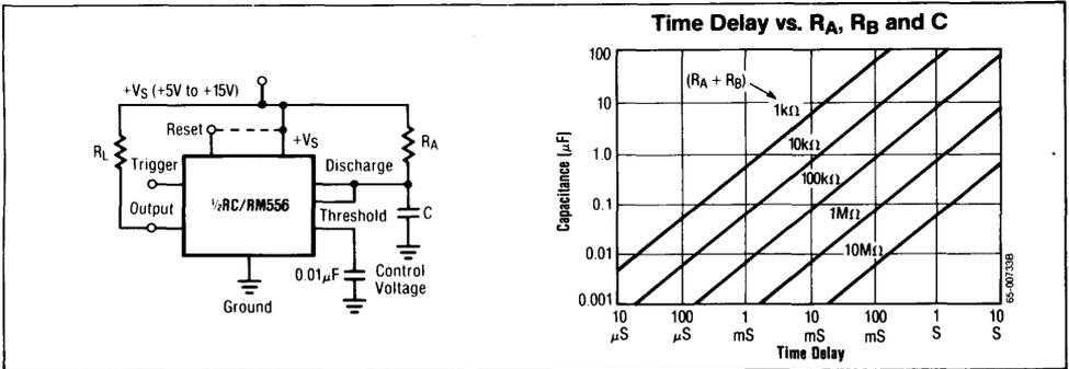
Figure 1. Monostable Operation
