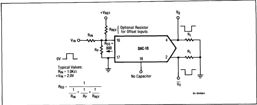
Figure 7. Pulsed Reference Operation
