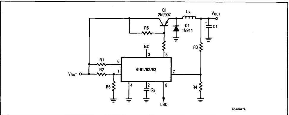
Figure 7. Step-Down Current Saver
