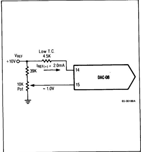
Figure 3. Recommended Full Scale Adjustment Circuit
