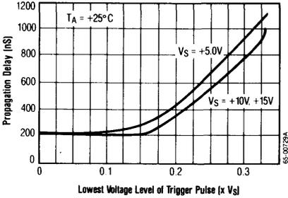
Output Propagation Delay vs. Voltage Level of Trigger Pulse
