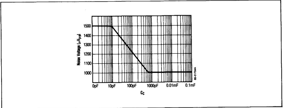
Figure 2. 0.1Hz ~ 1MHz Noise  $\mu\text{V}$  Peak-to-Peak Over 4 Second Scan
