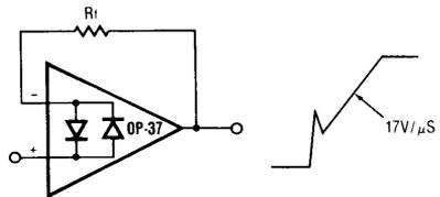
When  $R_i \leq 100\Omega$  and the input is driven with a fast, large signal pulse ( $\approx 1V$ ), the output waveform will look as shown
