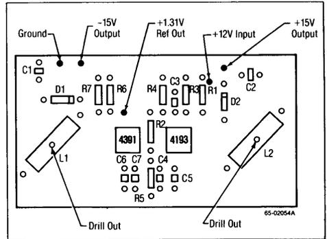
Figure 9. Dual Power Supply Component Placement Diagram
