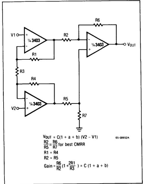
Figure 11. High Impedance Differential Amplifier
