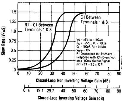
Slew Rate vs. Closed Loop Gain — 3078A
