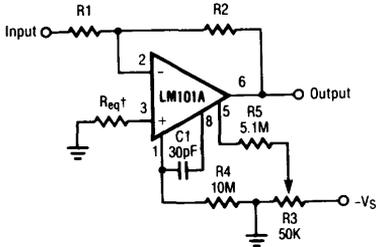
†May be zero or equal to parallel combination of R1 and R2 for minimum offset.
