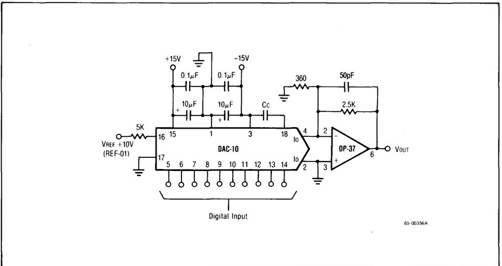
Figure 5. D/A Converter Application
