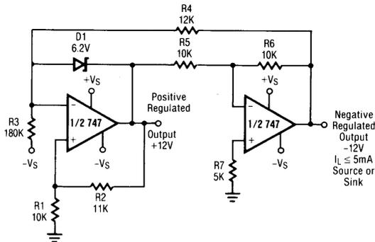
$$\text{Positive Output} = V_{D1} \times \frac{R1 + R2}{R2}$$
