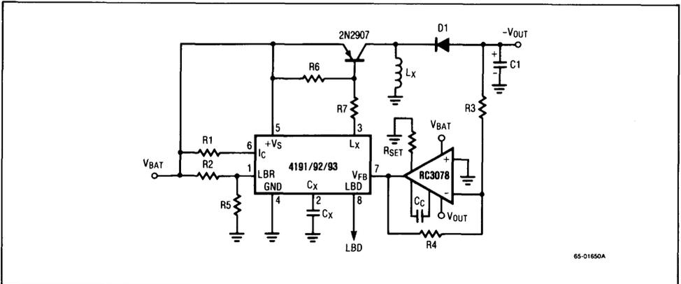
Figure 10. Inverting Switching Regulator Using 4191/92/93
