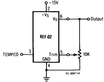
The REF-02 trim terminal can be used to adjust the output voltage over a 5V  $\pm 300mV$  range. This feature allows the system designer to trim system errors by setting the reference to a voltage other than 5V. Of course, the output can also be set to exactly 5.000V or to 5.12V for binary operation. Adjustment of the output does not significantly affect the temperature performance of the device. Typically the temperature coefficient change is 0.7ppm/ $^{\circ}C$  for 100mV of output adjustment.
