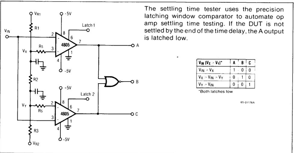
Figure 3. Precision Latching Window Comparator (Detail)
