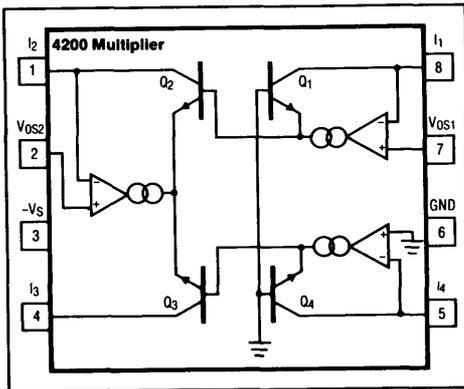
Figure 1. Functional Diagram
