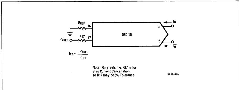
**Figure 4. Negative Reference Operation**
