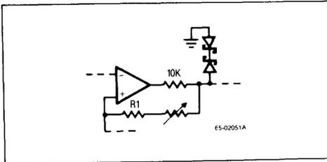
Figure 2. Triangle Generator — Symmetrical Output Option
