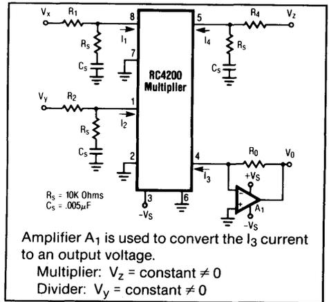
Amplifier A<sub>1</sub> is used to convert the I<sub>3</sub> current to an output voltage.
