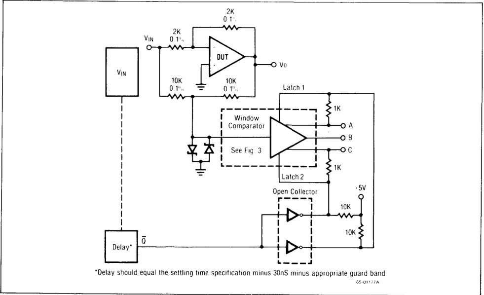
Figure 2. Op Amp Settling Time Tester
