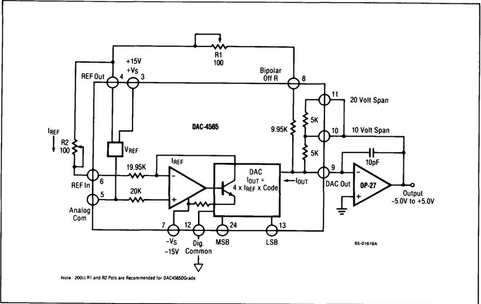
Figure 2. ±5.0V Bipolar Voltage Output
