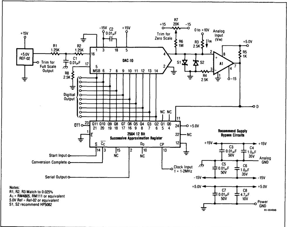
Figure 8. 10-Bit Successive Approximation A/D Converter
