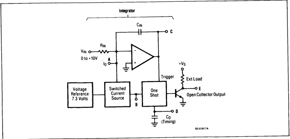
Figure 4. VFC Block Diagram
