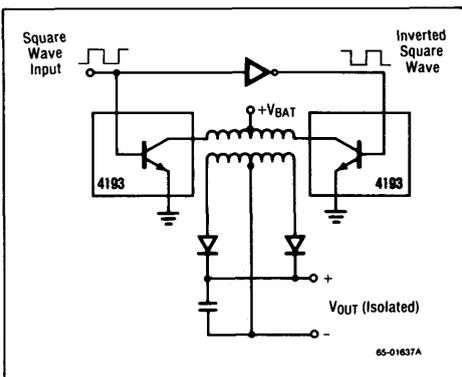
**Figure 21. Transformer Coupled Regulator
