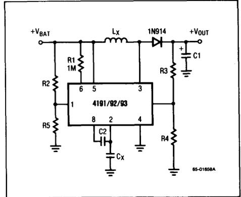
Figure 18. Step-Up Regulator With Voltage Dependent Oscillator
