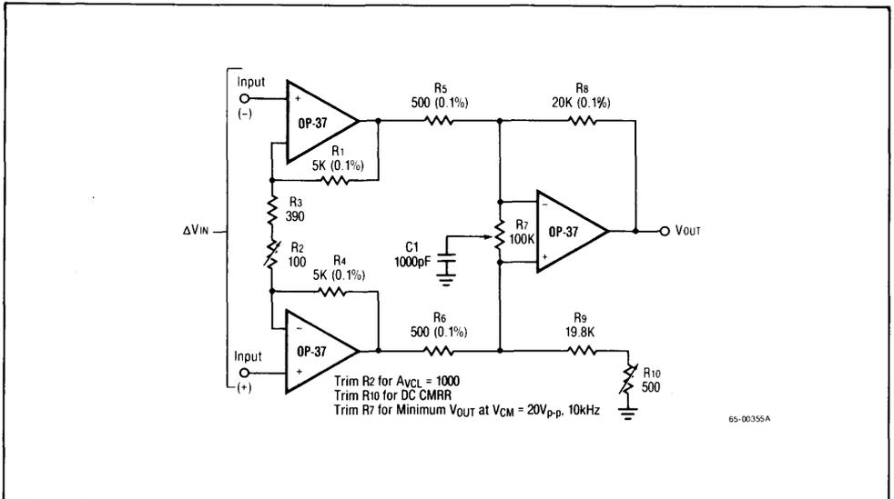
Figure 4. Three Op Amp IC Instrumentation Amplifier
