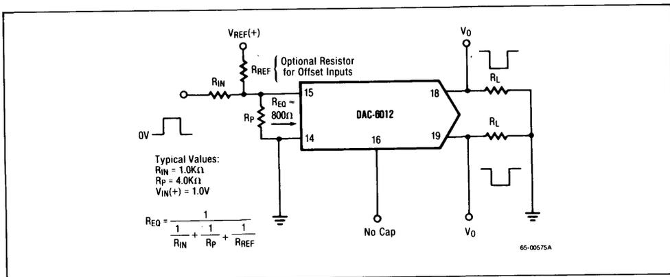
Figure 11. Pulsed Reference Operation
