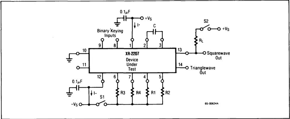
**Figure 1. Test Circuit for Split Supply Operation**
