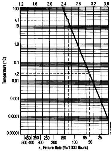
Figure 4. Failure Rate (1000/°K)
