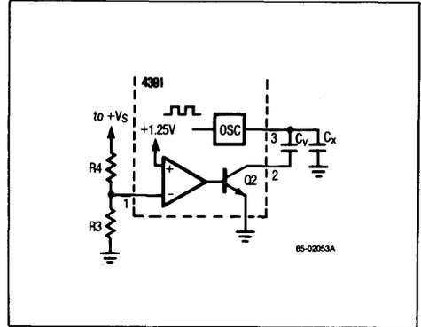
**Figure 6. Voltage Dependent Oscillator**
