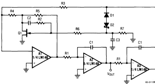
$$f = \frac{1}{2\pi R1C1} \times \sqrt{K}, K = \frac{R4R5}{R3} \left( \frac{1}{r_{DS}} + \frac{1}{R4} + \frac{1}{R5} \right), r_{DS} \approx \frac{R_{ON}}{\left(1 - \frac{V_{GS}}{V_P}\right)} \cdot 1/2$$
