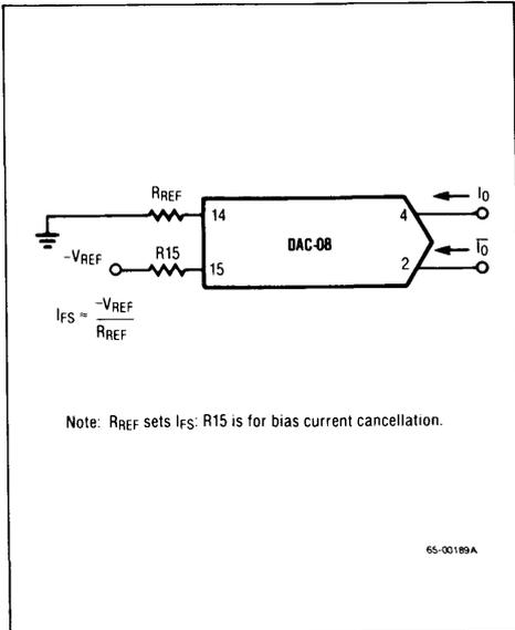
Figure 4. Basic Negative Reference Operation
