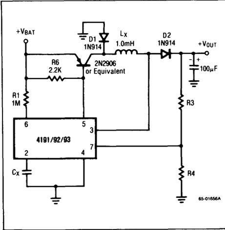
Figure 17. Buck Boost Circuit ( $V_{BAT} > \text{or} < V_{OUT}$ )
