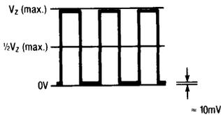
4. Return  $V_x$  (input) to ground and connect  $V_z$  (max.) DC on  $V_z$  (input). Adjust output  $V_{OS}(R_{17})$  for  $V_0 =$
