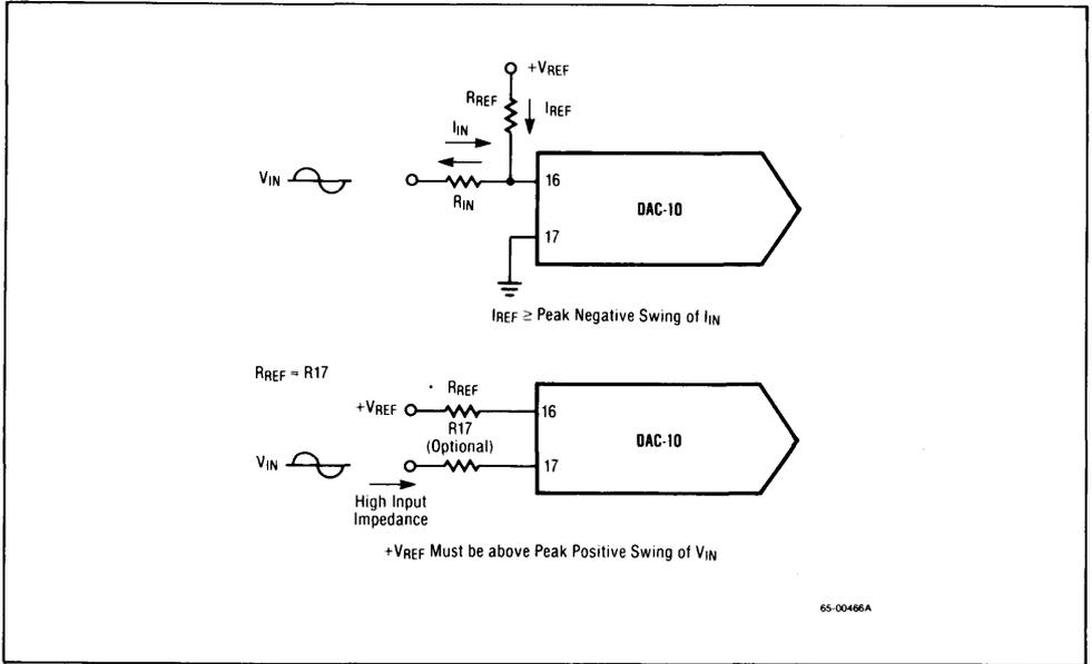
**Figure 5. Providing Offsets to Accommodate Bipolar References**
