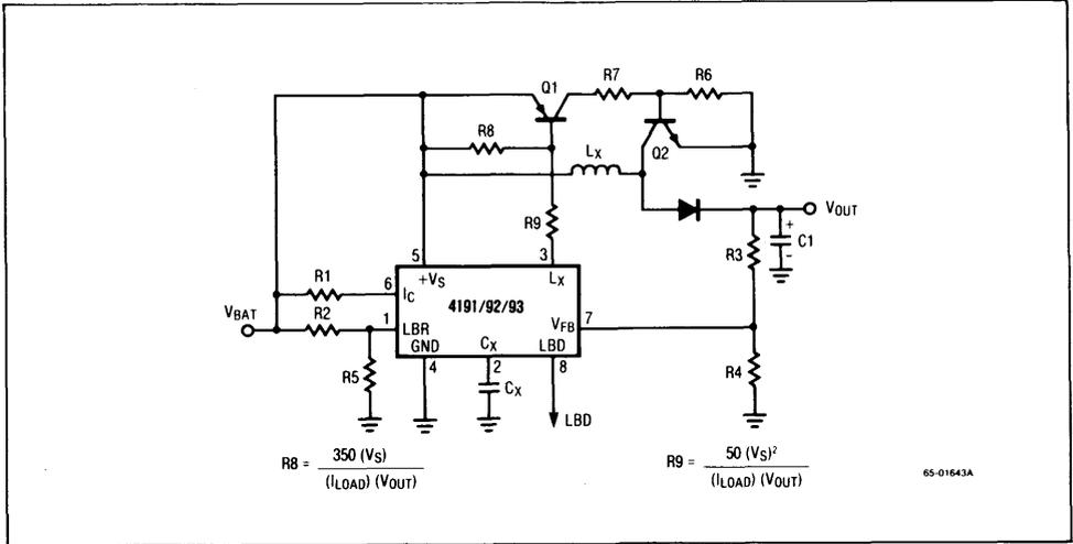
**Figure 4. Step-Up Switching Regulator (High Current)**
