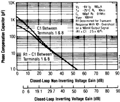
Phase Compensation Capacitance vs. Closed Loop Gain — 3078A
