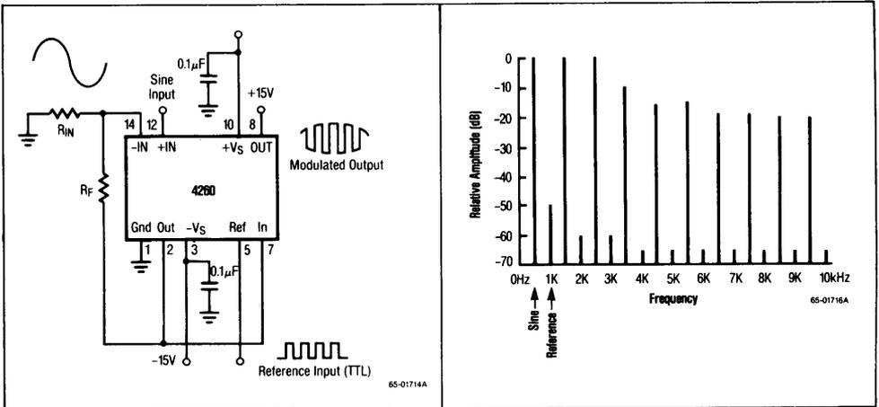
Figure 1. Suppressed Carrier Modulation
