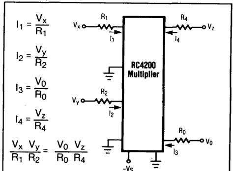
$$\text{Solving for } V_0: V_0 = \frac{V_x V_y R_0 R_4}{V_z R_1 R_2}$$
