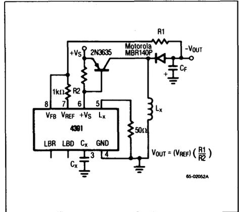
**Figure 4. High Current, High Efficiency Supply**
