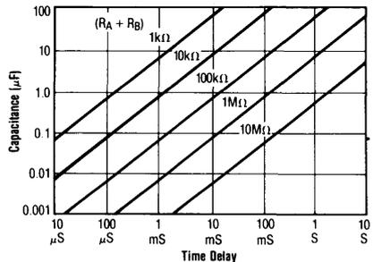
Figure 2. Monostable Operation
