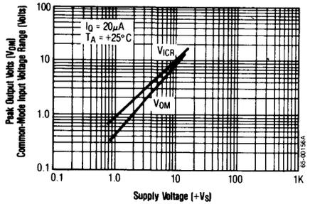
**Negative Output and Common Mode Voltage vs. Supply Voltage**
