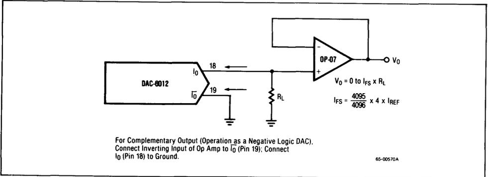
Figure 6. Positive Low Impedance Output Operations
