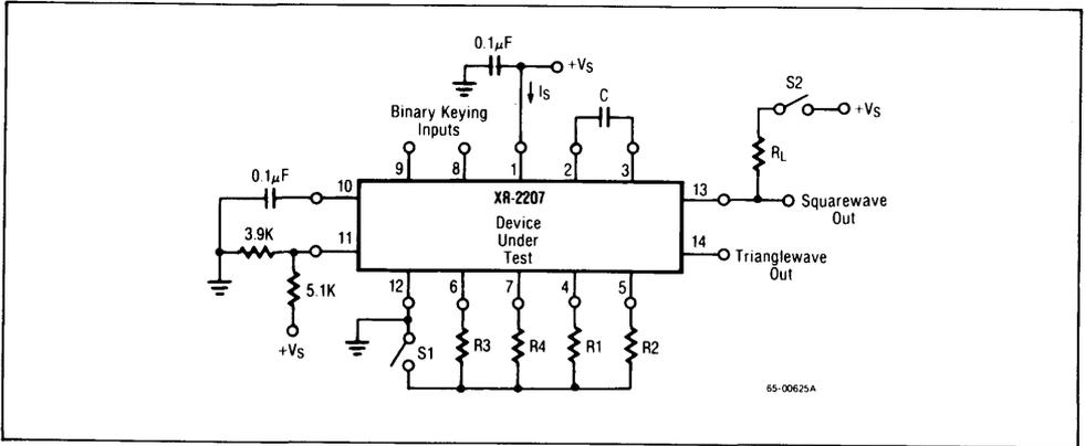
**Figure 2 Test Circuit for Single Supply Operation**
