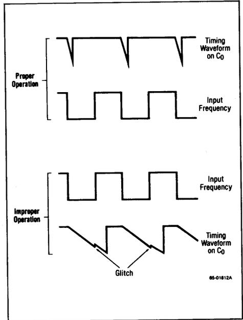
Figure 7. FVC Timing Waveform
