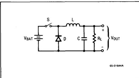
**Figure 5. Simple Step-Down DC-to-DC Converter ( $V_O \leq V_{BAT}$ )**
