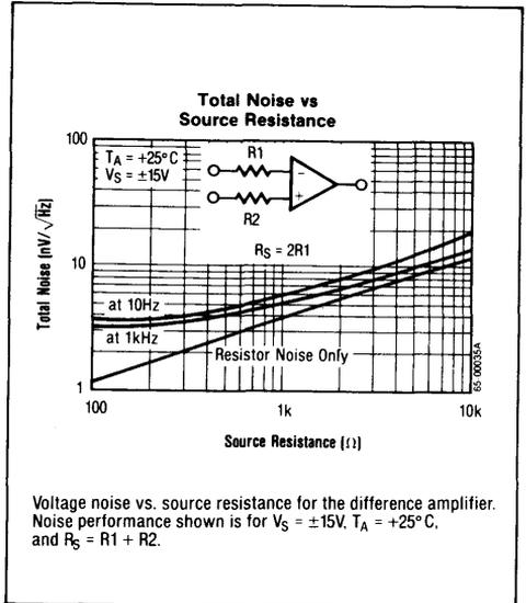
Voltage noise vs. source resistance for the difference amplifier. Noise performance shown is for  $V_S = \pm 15V$ ,  $T_A = +25^\circ C$ , and  $R_S = R_1 + R_2$ .
