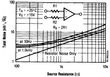
Voltage noise vs source resistance for the difference amplifier. Noise performance shown is for VS = ±15V, TA = +25°C, and RS = R1 + R2
