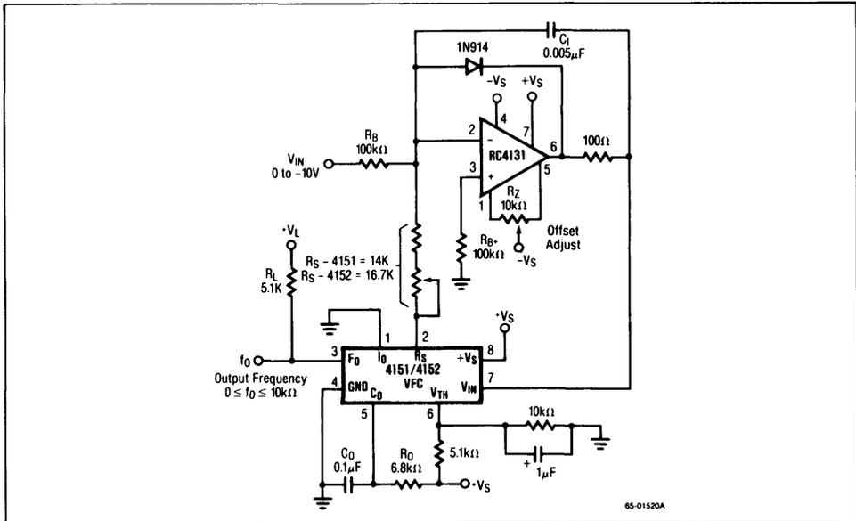
Figure 3. Precision Voltage — Sourced VFC
