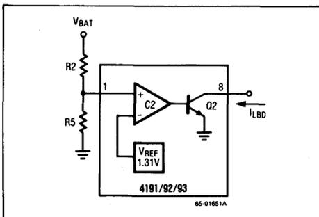
Figure 12. Low Battery Detector
