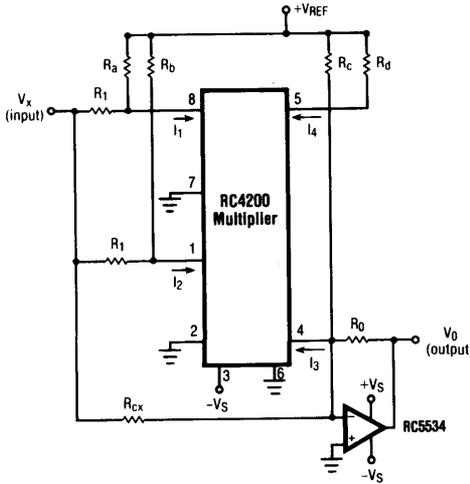
$$\frac{V_x^2}{R_1^2} + \frac{2V_x V_{REF}}{R_1 R_a} + \frac{V_{REF}^2}{R_a^2} = \frac{V_0 V_{REF}}{R_0 R_d} + \frac{V_{REF}^2}{R_c R_d} + \frac{V_x V_{REF}}{R_{cX} R_d}$$
