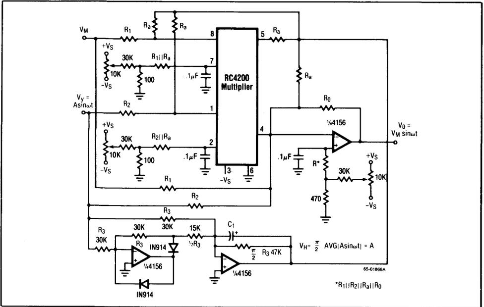
Figure 17. Amplitude Modulator with A.G.C.
