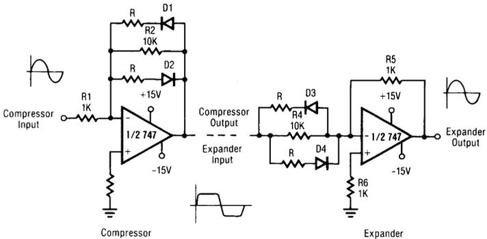
Maximum compression expansion ratio =  $R1/R$  ( $10K\Omega > R \geq 0$ )
