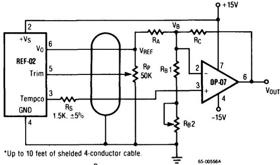
$$T_{C}V_{OUT} = (2.1mV/^{\circ}C) \left(1 + \frac{R_C}{R_A \parallel R_B}\right)$$
