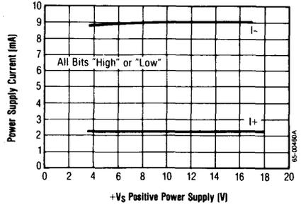
Power Supply Current vs. -V<sub>S</sub>
