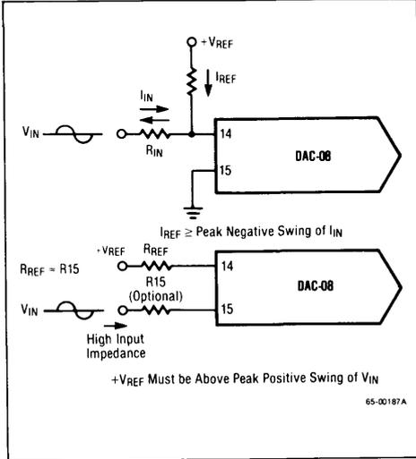
Figure 2. Accommodating Bipolar References
