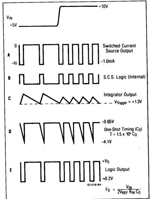
Figure 5. 4153 Voltage-to-Frequency Timing Waveforms
