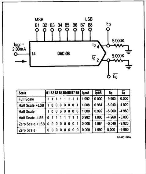
Figure 5. Basic Unipolar Negative Operation
