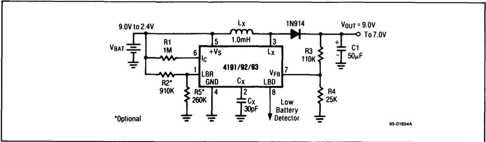
Figure 15. Typical Application: 9.0V Battery Life Extender
