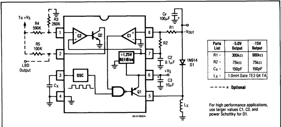
Figure 2. 4391 Standard Application Circuit
