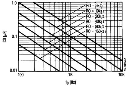
VCO Frequency vs. Timing Capacitor
