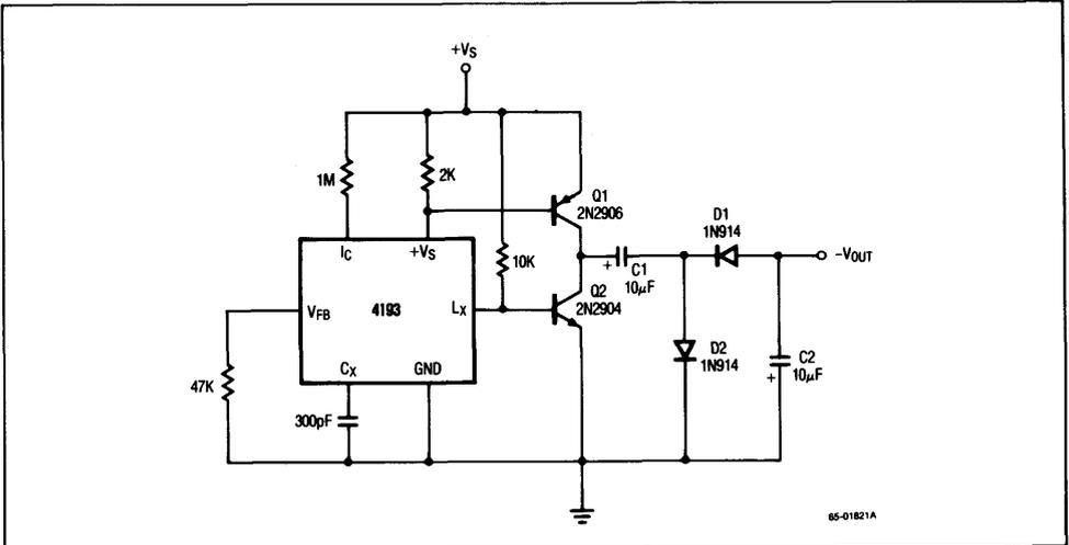
**Figure 20. Inductorless Inverter**
