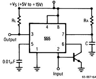
Figure 1. Missing Pulse Detector
