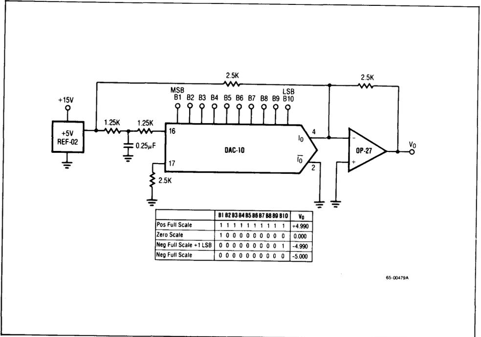
Figure 16. Offset Binary Operation
