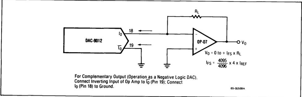
Figure 5. Negative Low Impedance Output Operations
