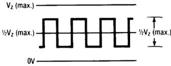
3. Connect  $V_x$  (input to  $V_z$  (input) and put in the  $\frac{1}{2}V_z$  (max.) DC with an AC of approximately 20mV less than  $V_z$  (max.).
