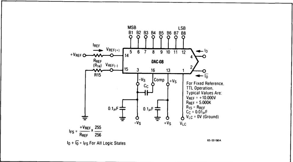
Figure 1. Basic Positive Reference Operation
