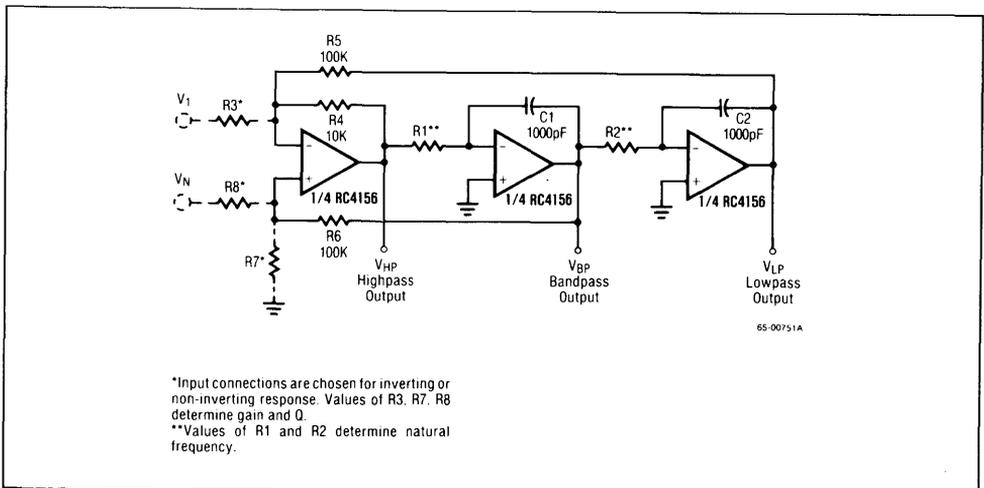
Figure 3. Generalized State-Variable Configuration for Active Filter
