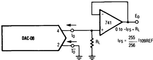
For complementary output (operation as a negative logic DAC), connect non-inverting input of Op-Amp to  $I_0$  (pin 2); connect  $I_0$  (pin 4) to ground.
