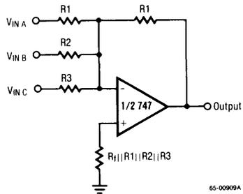
$$-V_O = V_{IN A} \left( \frac{R_1}{R_1} \right) - V_{IN B} \left( \frac{R_1}{R_2} \right) - V_{IN C} \left( \frac{R_1}{R_3} \right)$$
