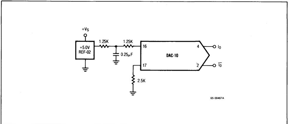
**Figure 6. Input Reference Noise Limiting Filter**
