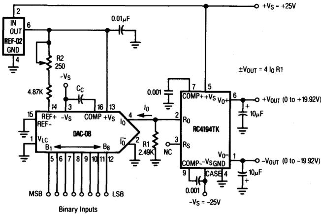
Adjust R2 for -19.92V at -VOUT with all "1"s at binary inputs, then optionally adjust R3 for +19.92V at +VOUT
