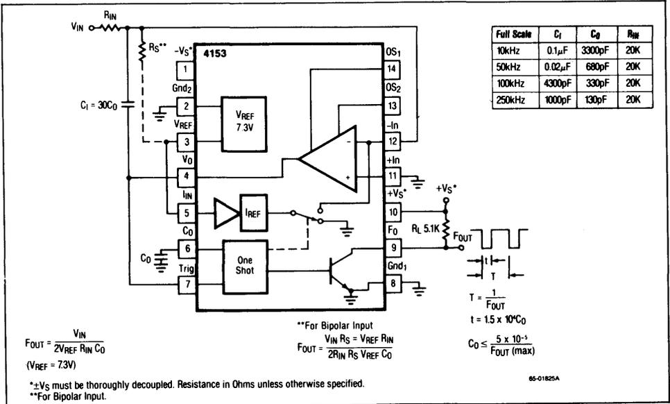
Figure 1. Voltage-to-Frequency Converter Minimum Circuit
