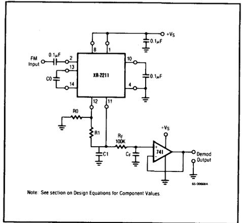
**Figure 5. Linear FM Detector Using XR-2211 and an External Op Amp**
