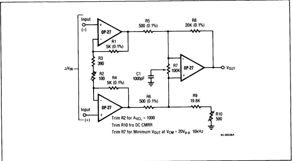
Figure 8. Three Op Amp IC Instrumentation Amplifier
