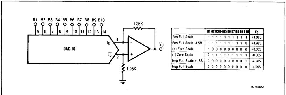
Figure 2. Bipolar Operation
