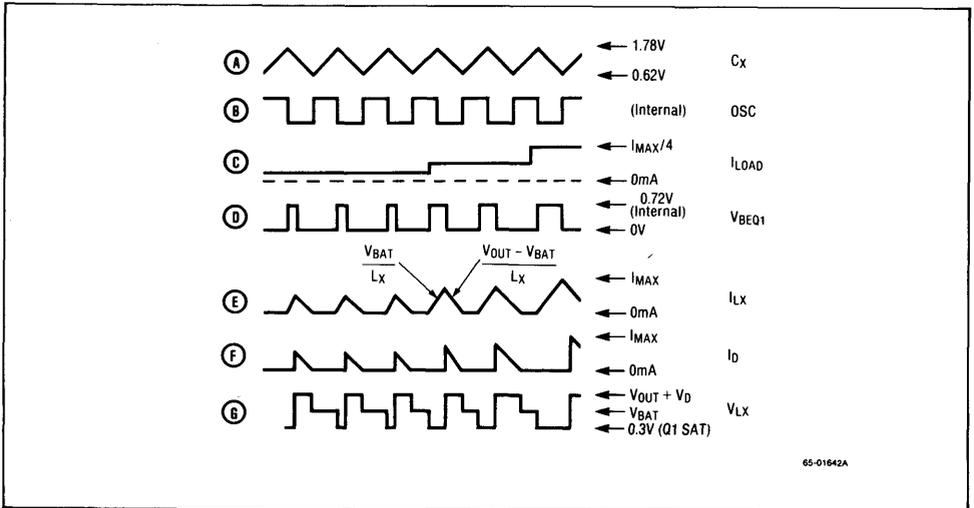
Figure 3. Step-Up Regulator Waveforms
