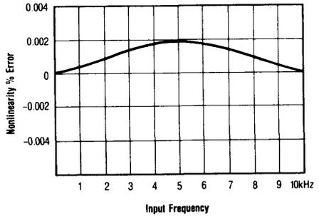
4153 50kHz Voltage-to-Frequency Nonlinearity
