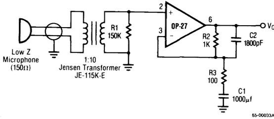
Figure 3. Low Impedance Microphone Preamplifier
