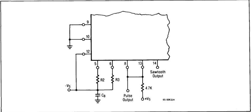
Figure 4. Pulse and Sawtooth Generation
