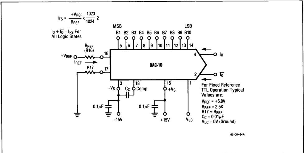
**Figure 3. Positive Reference Operation**
