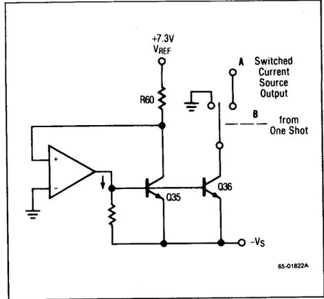
Figure 10. Switched Current Source Simplified Diagram
