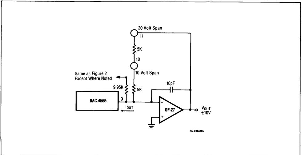
Figure 3. ±10V Bipolar Voltage Output
