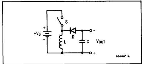
Figure 1. Simplified Voltage Inverter
