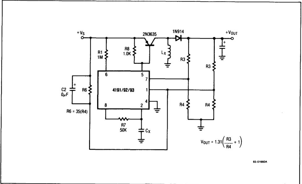
Figure 19. Step-Down Regulator With Short Circuit Protection
