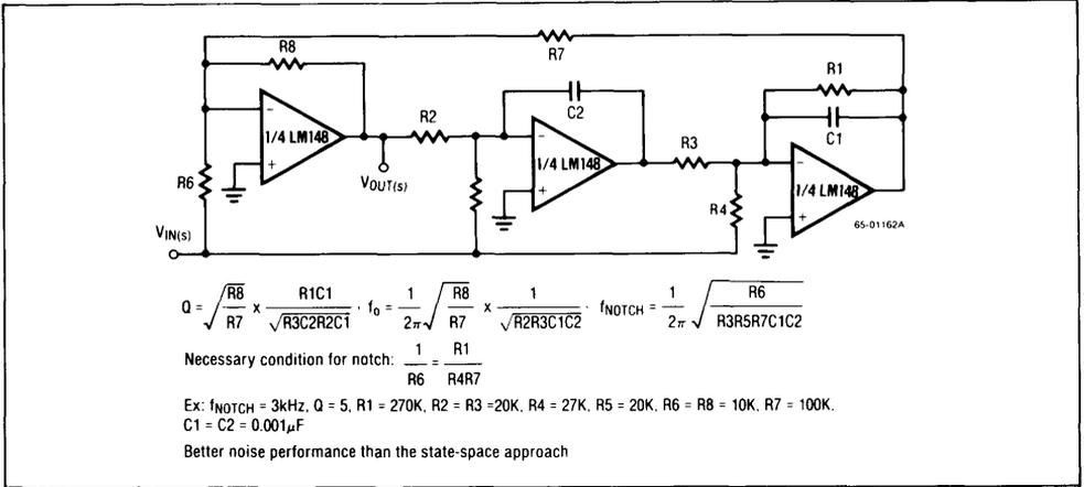
Figure 7. 3 Amplifier Bi-Quad Notch Filter
