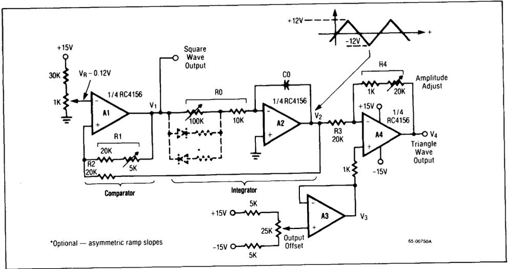
Figure 1. Triangle and Square Wave Generator
