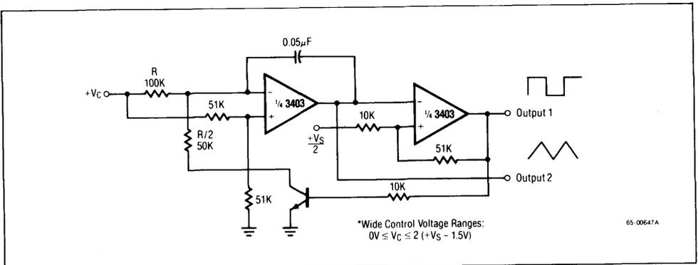
Figure 6. Voltage Controlled Oscillator
