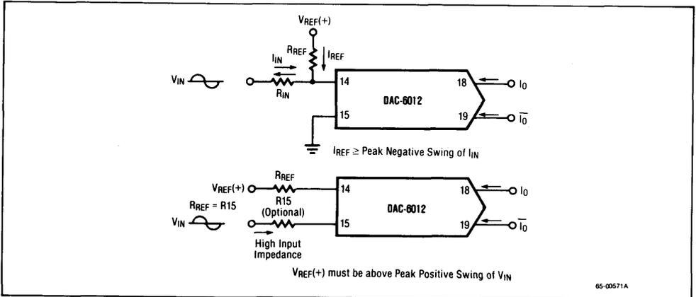
Figure 7. Accommodating Bipolar References
