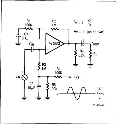
Figure 7. AC Coupled Non-Inverting Amplifier
