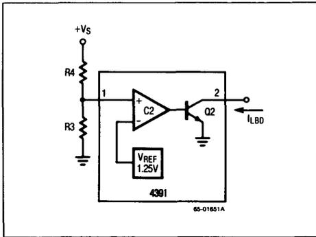
**Figure 3. Low Battery Detector**
