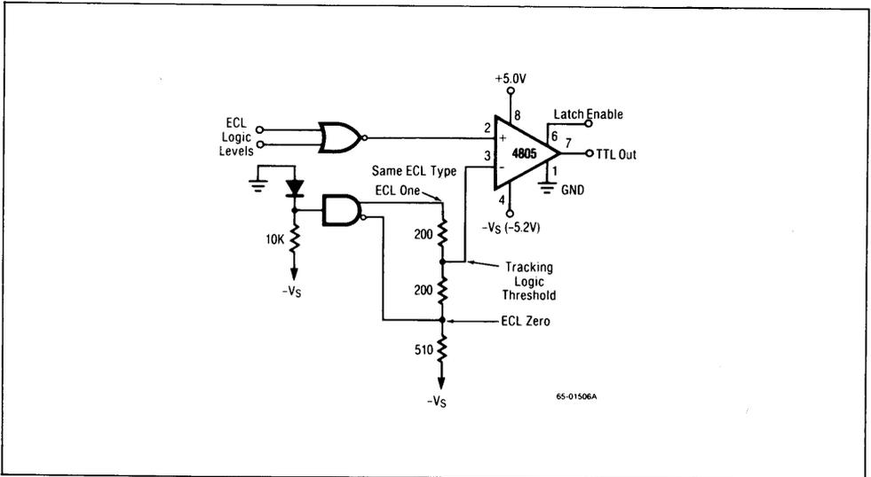
Figure 6. Single-Ended ECL to TTL Translator with Tracking ECL Reference
