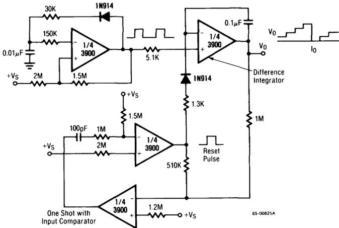
**Supplying  $I_{IN}$  With Auxiliary Amplifier
