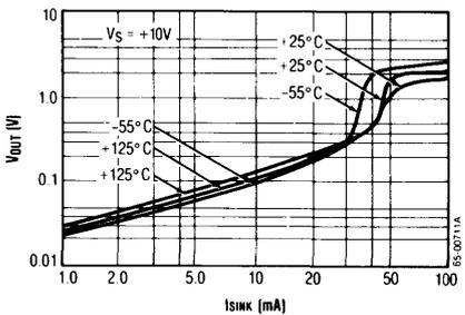
Low Output Voltage vs. Output Sink Current
