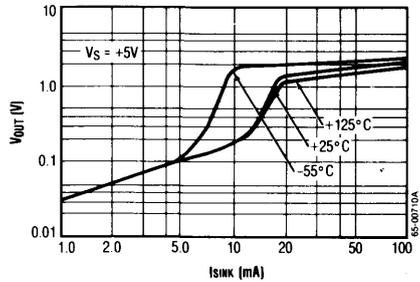
Low Output Voltage vs. Output Sink Current
