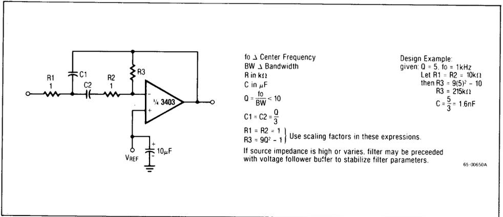
Figure 9. Multiple Feedback Bandpass Filter
