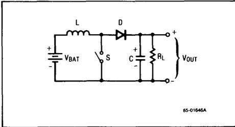
**Figure 1. Simple Step-Up DC-to-DC Converter**
