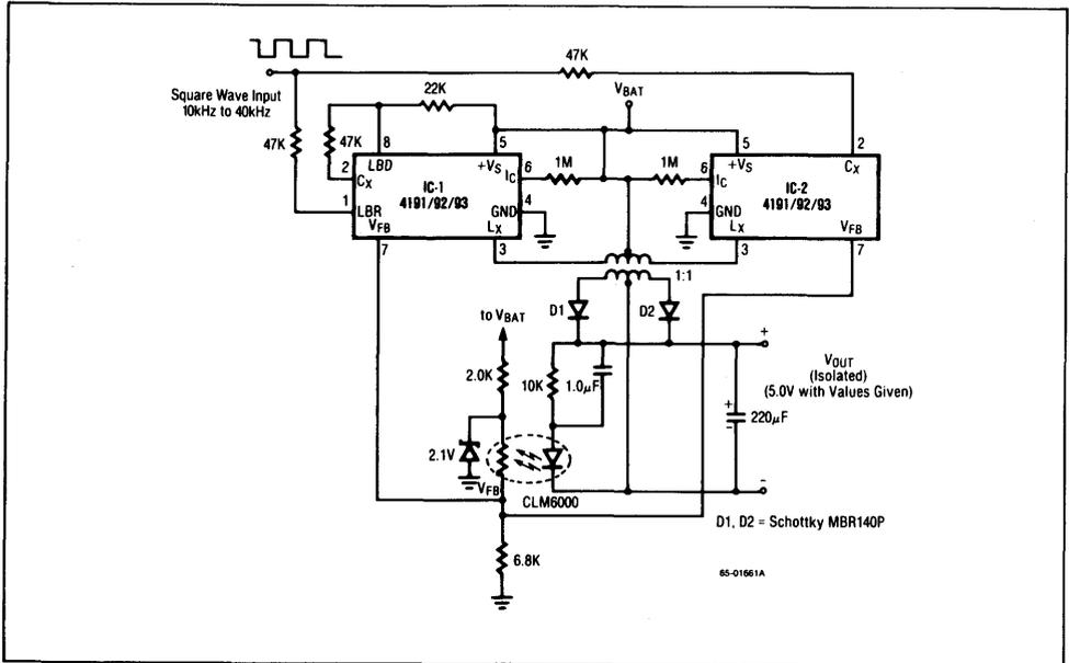
**Figure 22. Isolated Push-Pull Transformer Coupled Regulator**
