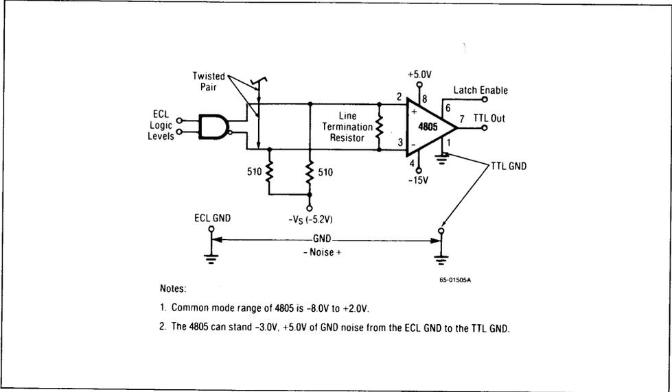
Figure 5. ECL to TTL Translator with Extended Common Mode Range
