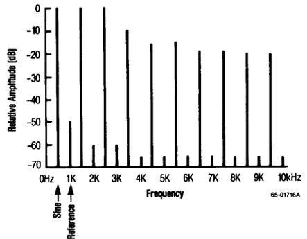
Figure 2. Spectral Plot ( $V_{IN} = 500\text{Hz}$ , TTL Ref = 1kHz)
