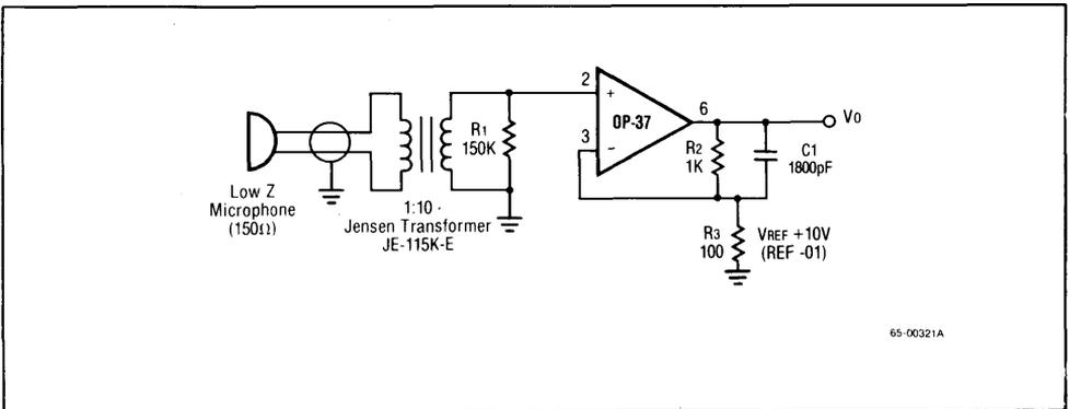
Figure 1. Low Impedance Microphone Preamplifier
