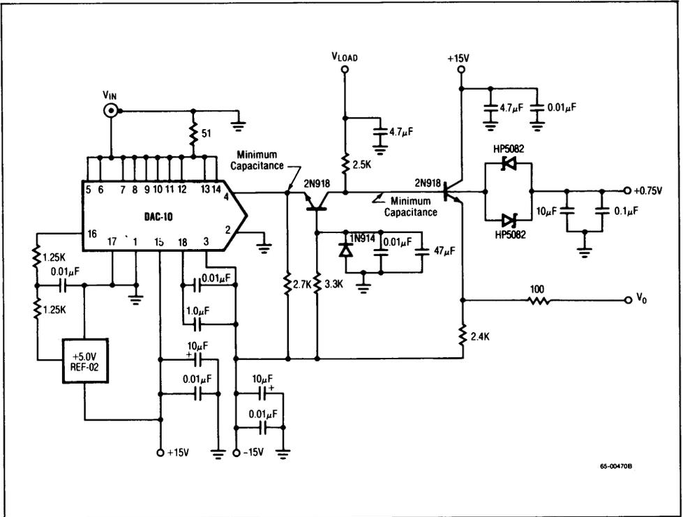
Figure 1. Settling Time Test Fixture
