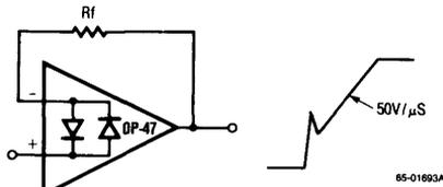
When  $R_f \leq 100\Omega$  and the input is driven with a fast, large signal pulse ( $\geq 1V$ ), the output waveform will look as shown.
