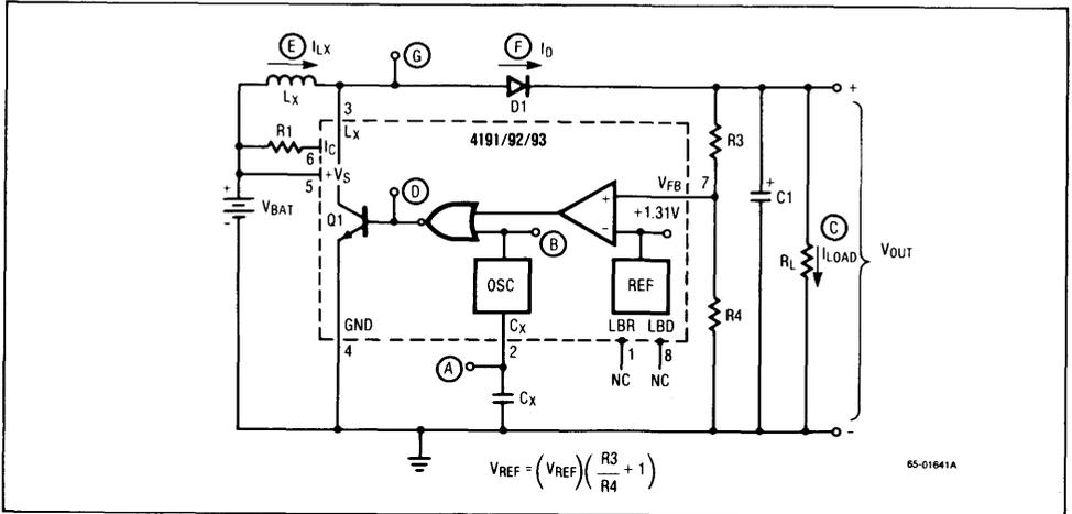
Figure 2. Minimum Step-Up Application
