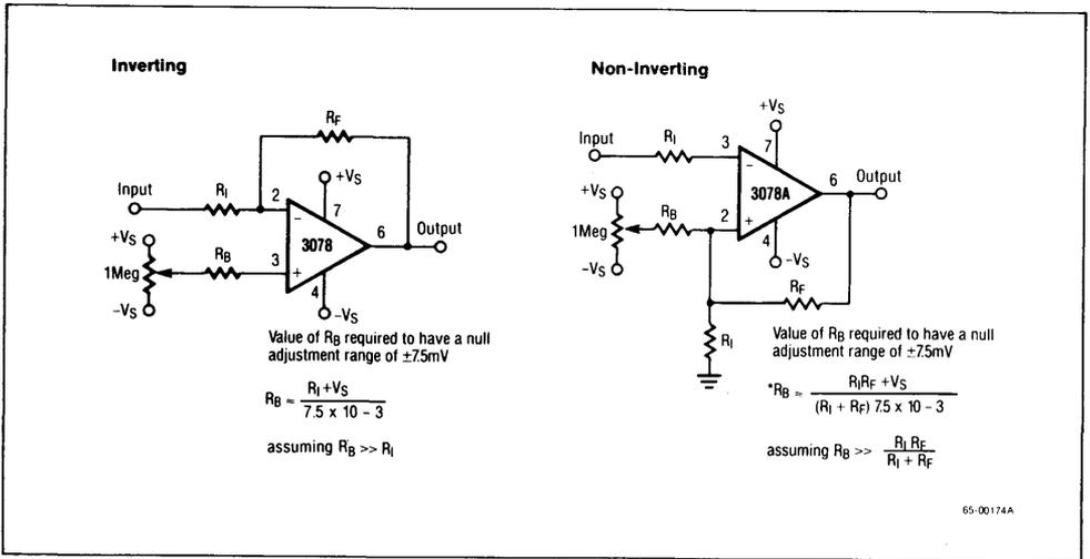
**Figure 1. Offset Voltage Null Circuit**
