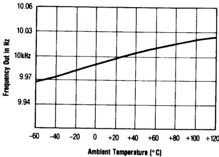
4153 250kHz Full Scale Temperature Drift
