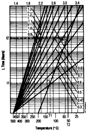
Figure 3. Normalized Time-Temperature Regressions for Various Activation Energy Values (1000/°K)
