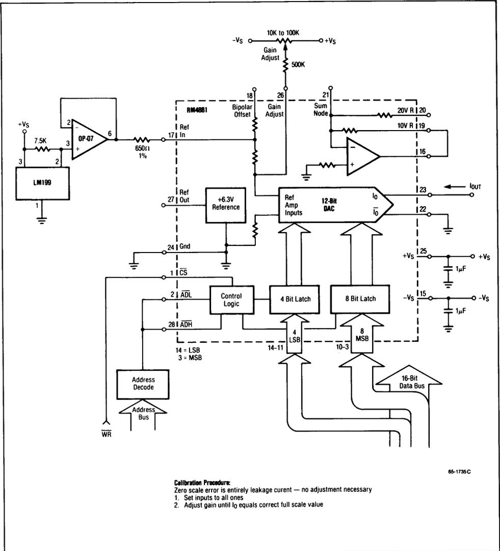
**Figure 8. Microprocessor Interface, 16-Bit Data Bus, 0 to -4mA Output
