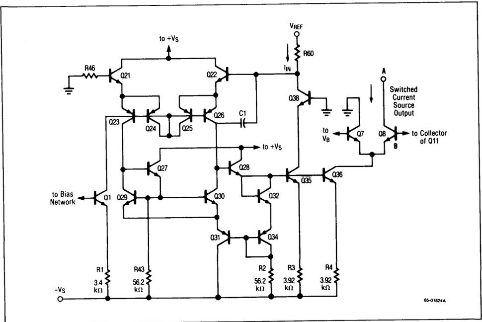
Figure 11. Switched Current Source (Detail)
