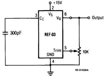
The REF-03 trim terminal can be used to adjust the output voltage over a  $2.5V \pm 150mV$  range. This feature allows the system designer to trim system errors by setting the reference to a voltage other than 2.5V. Of course, the output can also be set to exactly 2.500V or to 2.56V for binary operation. Adjustment of the output does not significantly affect the temperature performance of the device. Typically the temperature coefficient change is 0.7ppm/°C for 100mV of output adjustment.
