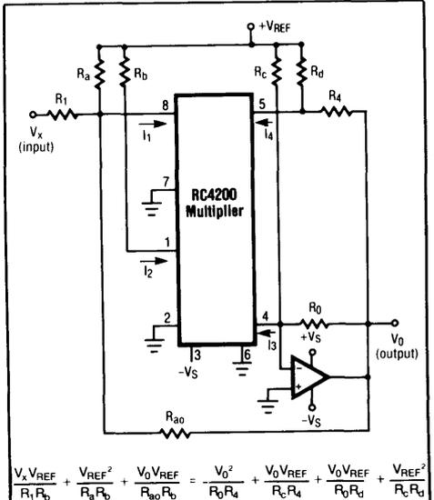
$$\frac{V_x V_{REF}}{R_1 R_b} + \frac{V_{REF}^2}{R_b R_b} + \frac{V_0 V_{REF}}{R_{a0} R_b} = \frac{V_0^2}{R_b R_4} + \frac{V_0 V_{REF}}{R_c R_4} + \frac{V_0 V_{REF}}{R_0 R_d} + \frac{V_{REF}^2}{R_c R_d}$$
