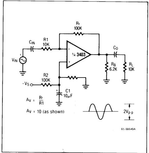
Figure 8. AC Coupled Inverting Amplifier
