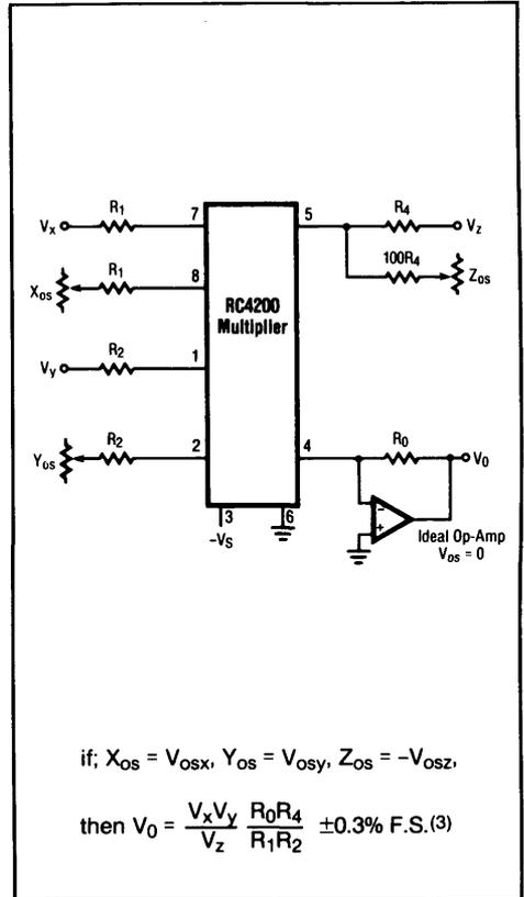
Figure 14. 4200 With Input Offset Adjustment
