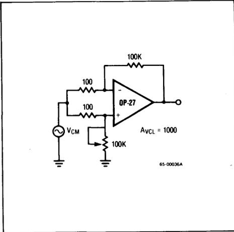
Figure 6. Common Mode Rejection Ratio Test Circuit
