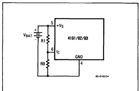
Figure 13. Simple Automatic Shutdown
