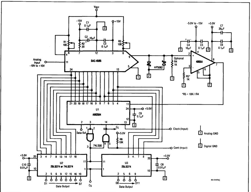
Figure 7. 12-Bit Analog-to-Digital Converter
