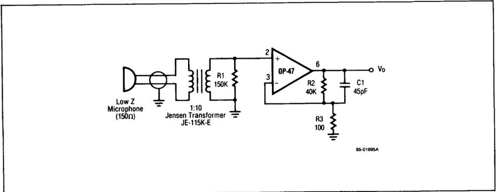
Figure 1. Low Impedance Microphone Preamplifier
