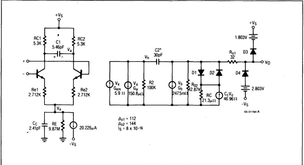
Figure 1. LM148 Macromodel for Computer Simulation
