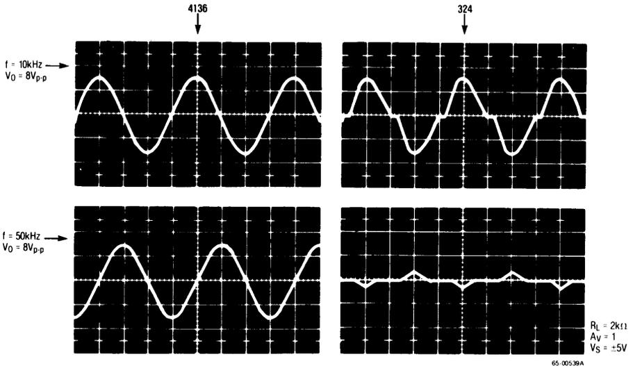
Output Voltage Swing as a Function of Frequency
