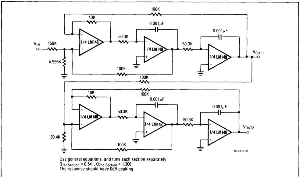
Figure 6. 1kHz 4 Pole Butterworth Filter
