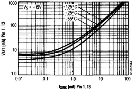
Discharge Transistor (Pin 1, 13) Voltage vs. Sink Current
