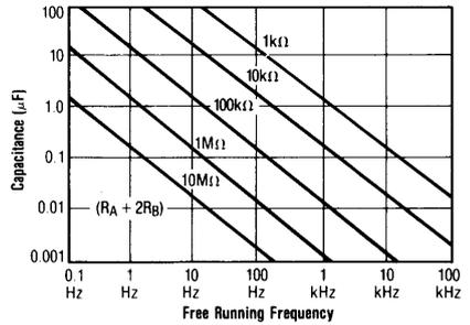
**Figure 3. Free Running Operation**
