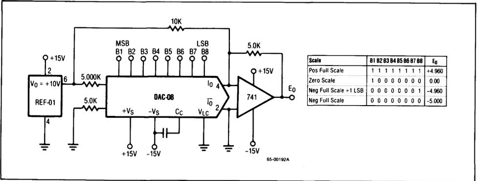
Figure 7. Offset Binary Operation
